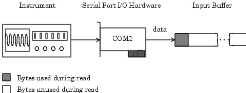
Note that for a given read operation, you might not know the number of bytes returned by the device. Therefore, you might need to preset the `InputBufferSize` property to a sufficiently large value before connecting the serial port object.
