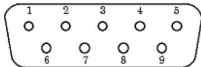
The pins and signals associated with the 9-pin connector are described in the following table. Refer to the RS-232 standard for a description of the signals and pin assignments used for a 25-pin connector.
