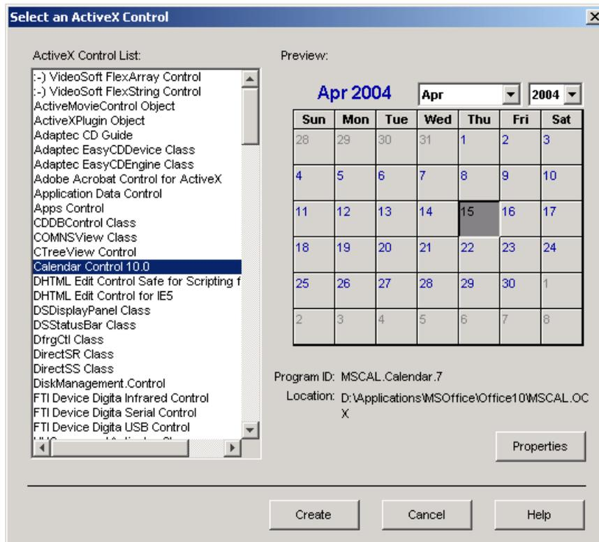
The interface has an **ActiveX Control List** selection pane on the left and a **Preview** pane on the right. To see a preview of the control, click one of the control names in the selection pane. (A blank preview pane means that the control does not have a preview.) If MATLAB cannot create the instance, an error message appears in the preview pane.
