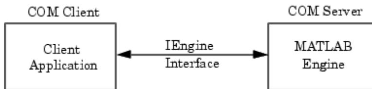
Use the MATLAB Engine API functions to start and end the server process, and to send commands to be processed by MATLAB.
