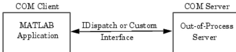
As with in-process servers, this server exposes its properties and methods through the IDispatch (Automation) interface or a Custom interface, depending on which interfaces the component implements. For information on accessing interfaces, see “COM Object Interfaces” on page 12-32.
