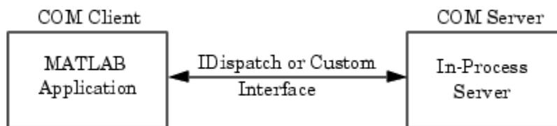
The server exposes its properties and methods through the IDispatch (Automation) interface or a Custom interface, depending on which interfaces the component implements. For information on accessing interfaces, see “COM Object Interfaces” on page 12-32 .
