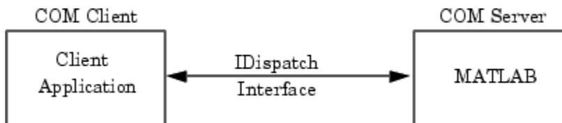
MATLAB Automation server capabilities include the ability to execute commands in the MATLAB workspace, and to get and put matrices directly from and into the workspace. You can start a MATLAB server to run in either a shared or dedicated mode. You also have the option of running it on a local or remote system.
