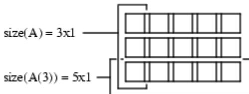
`size(A)` returns the dimensions of the highest array level of `A`. The highest level of the array has a size of 3-by-1.
